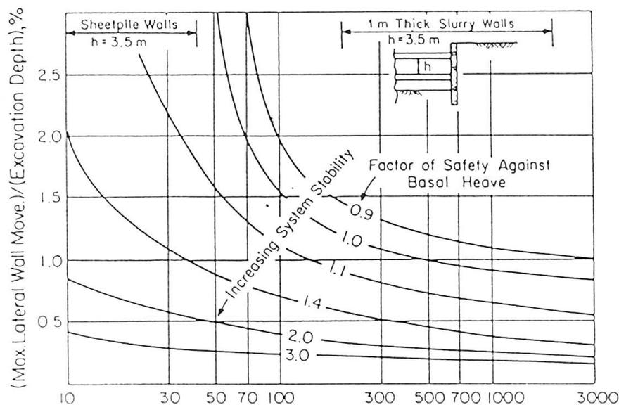
The figure and accompanying study were prepared by correlating soil-structure interaction analyses to wall movement calculations observed from actual excavations.
