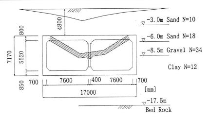
Fig. -1.1 Damages at Daikai Station
