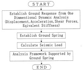
Fig. -3.2 Flow Diagram of Seismic Deformation Method
