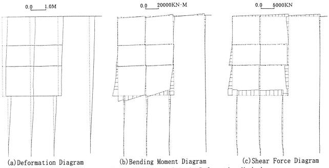
Fig. -7.2 Result of Non-linear Seismic Deformation Method
