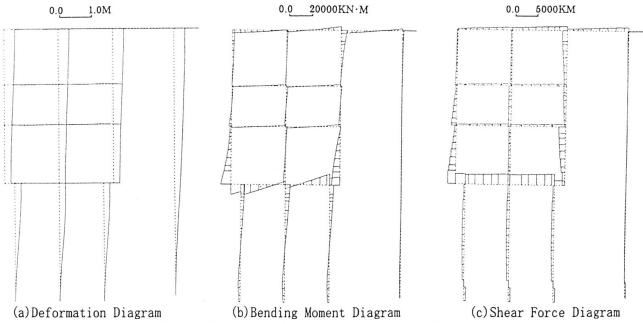
Fig. -5.3 Result of Seismic Deformation Method
