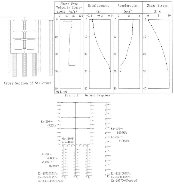
Fig. -5.2 Model of Seismic Deformation Method
