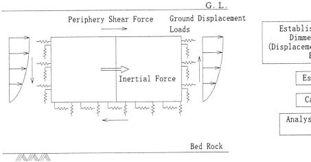
Fig. -3.1 The Concept of Seismic Deformation Method
