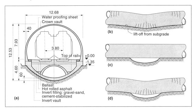
Fig. 2 Typical cross-section of the tunnel (a), fundamental cases of structural performance: extensive long term subsidence (b), doline (c) and subsidence with doline (d)
