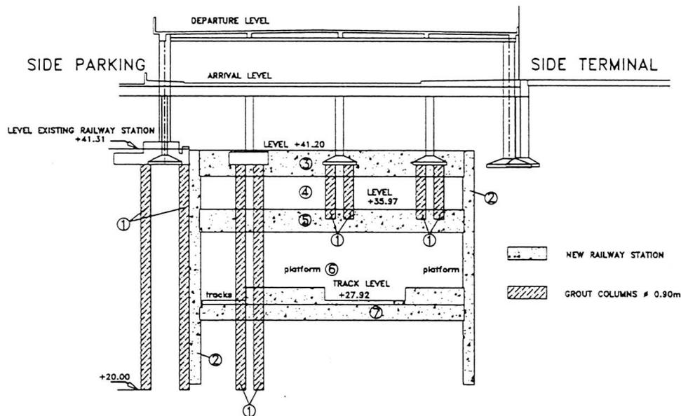
1. Execution of V.H.P.-columns after the boring of pits throughout the existing foundation soles.
