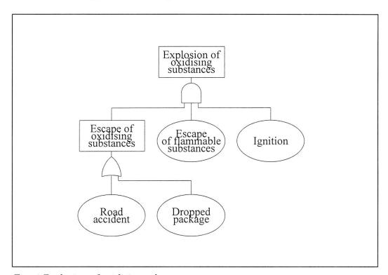
Fig. 4 Explosion of oxidising substances
