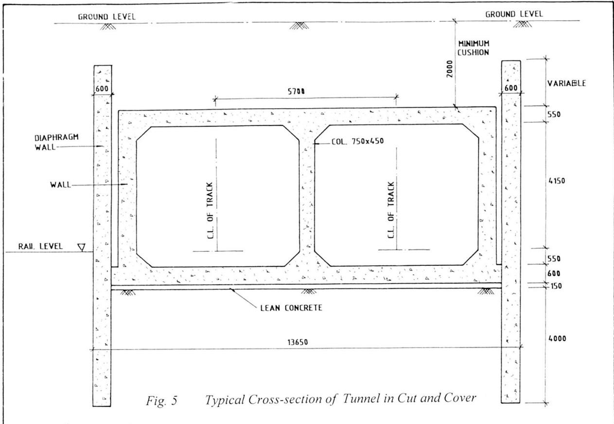
Fig. 5 Typical Cross-section of Tunnel in Cut and Cover
