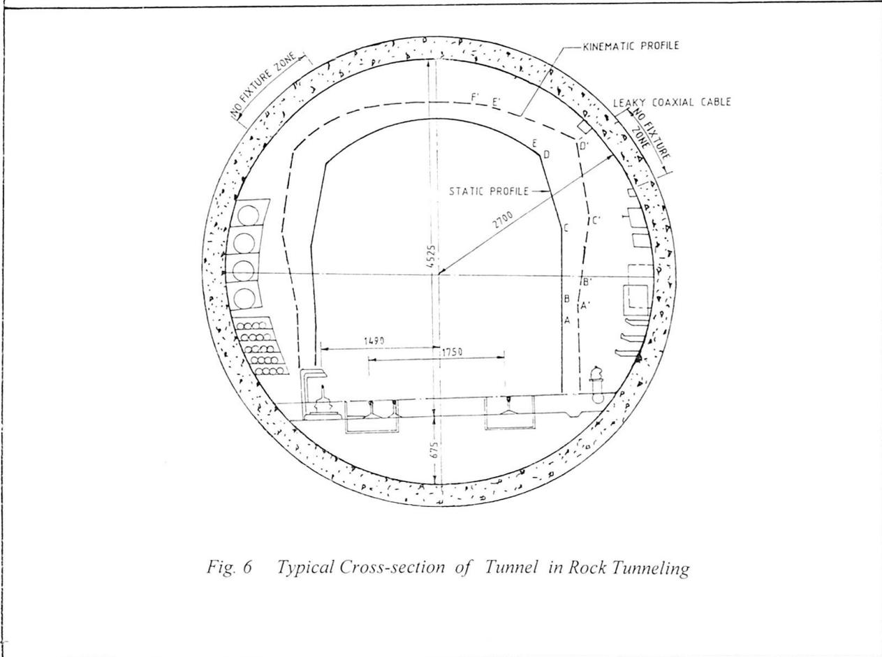
Fig. 6 Typical Cross-section of Tunnel in Rock Tunneling
