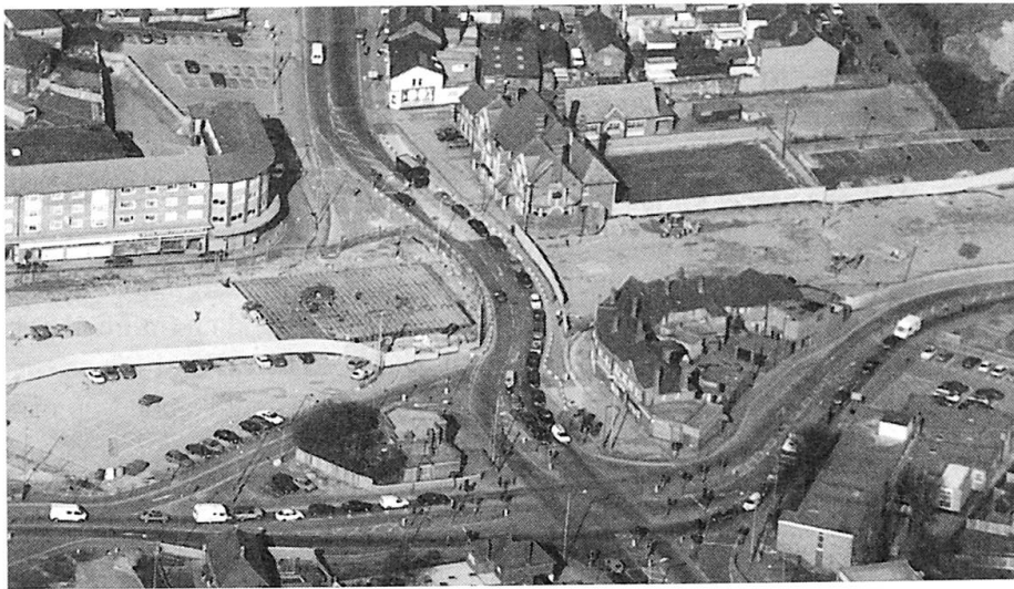
Figure 2: Road diversion during tunnel construction
