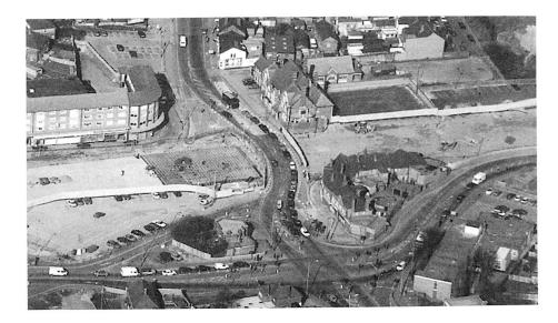
Figure 2: Road diversion during tunnel construction
