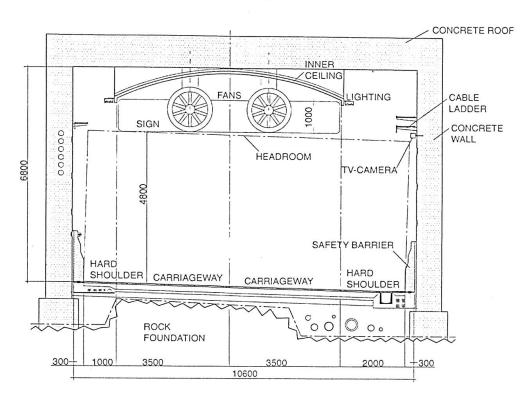
Fig. 4 Concrete Tunnel Section
