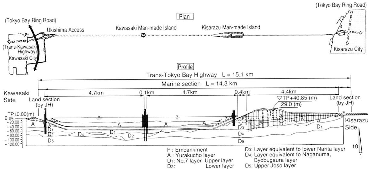
Fig. 2 Project plan and geological profile
