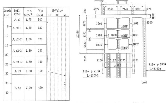
Fig.-2.1 Cross Section View of Yokohama MM21 Line Underground Station
