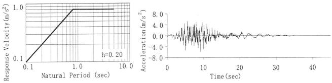
Fig. -4.1 Response Velocity Spectrum
