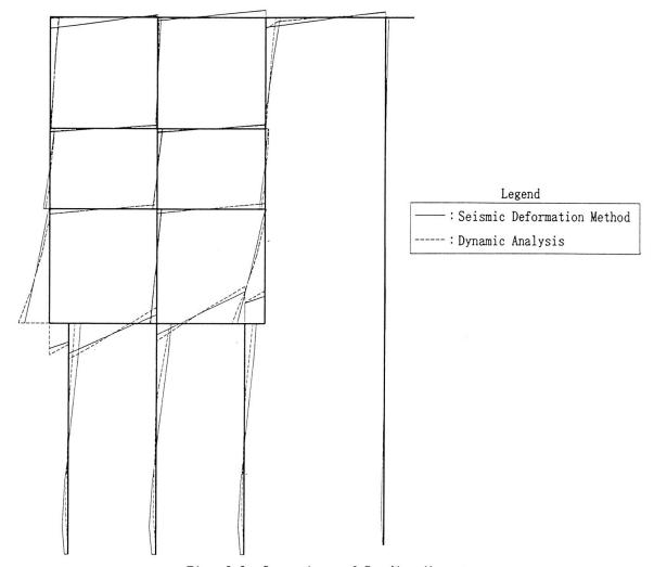
Fig. -6.3 Comparison of Bending Moment
