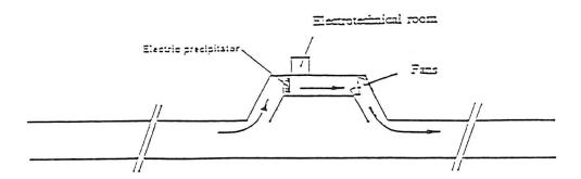
Fig. 2 The principle for a bypass solution selected in the Granfoss Tunnel and the Ekeberg Tunnels
