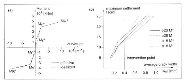
Fig. 4 Moment-curvature diagram for rebars Ø 26 mm (a) and settlement - crack width diagram for standard subsidence shape 1 (b)
