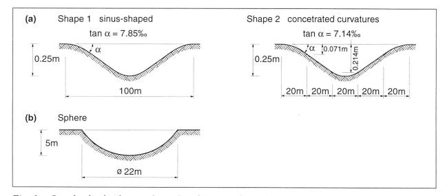
Fig. 1 Standard subsidences shape 1 and 2 (a) and standard doline (b)
