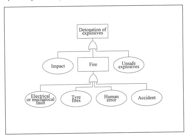
Fig. 3 Detonation of explosives
