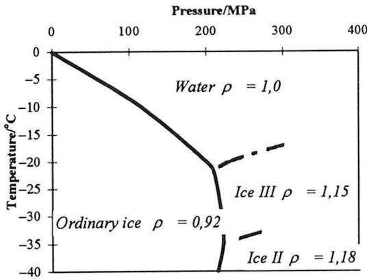
Figure 1 Relation between temperature and pressure and ice formation.
