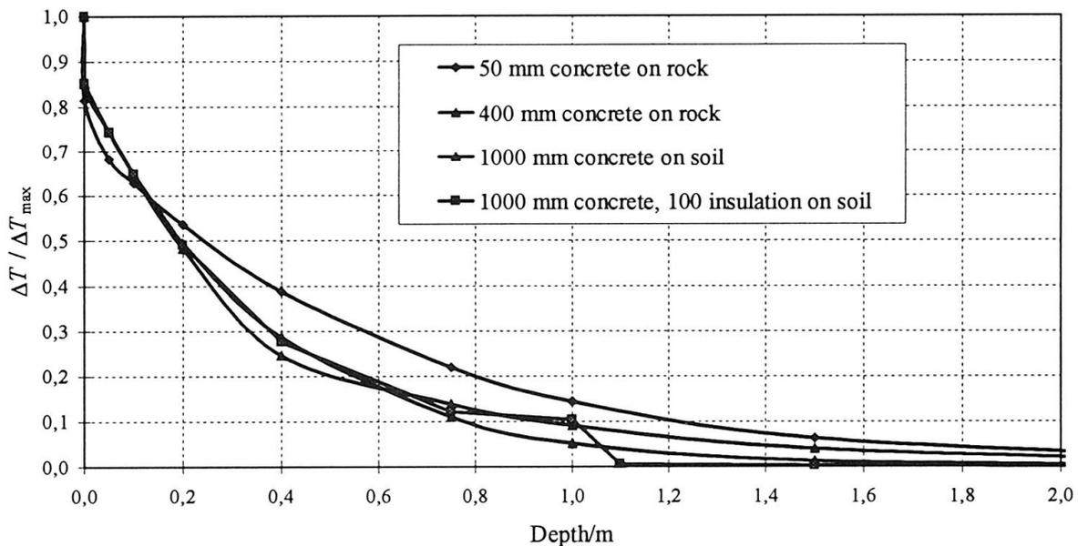
Figure 5 Temperature variation  $\Delta T$  at different depths in a lining when the temperature is varied with a period of one week with the amplitude  $\Delta T_{\max}$ .
