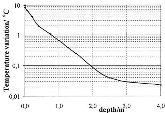
*Figure 6* Temperature penetration when the outer temperature varies in 6 day cycles (+4°C to -6°C) for a 400 mm concrete lining on rock.
