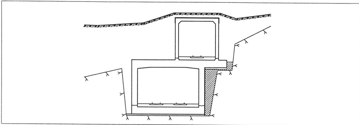
*Fig 1 : Fly-over tunnels below the Märsta River*
