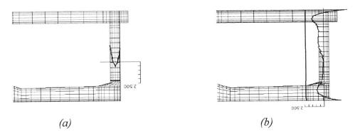
Figure 3. a) Longitudinal stress profile in outer wall at the concrete core after 504 hours. b) Stress profile in plane of cross section in the outer wall after 504 hours.
