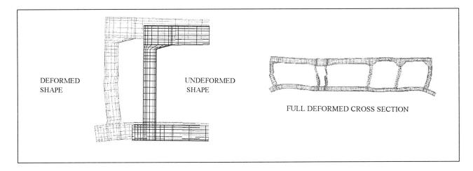
Figure 2. Distorted shape of tunnel cross-section due to temperature evolution.
