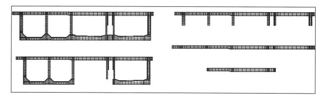
Figure 1. Finite element model for stress and temperature analysis, built up in stages corresponding to the casting sequence.
