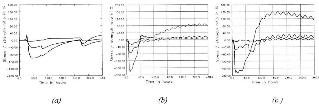
Figure 4. a) Risk of cracking for full section casting 1.0m above base slab in outer wall.
