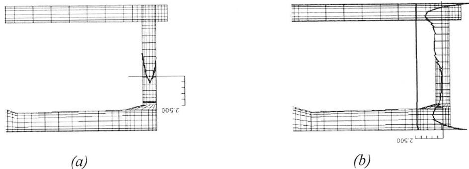
Figure 3. a) Longitudinal stress profile in outer wall at the concrete core after 504 hours.
