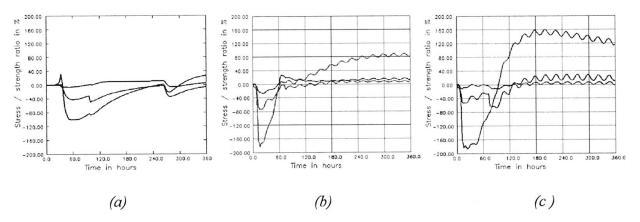
Figure 4. a) Risk of cracking for full section casting 1.0m above base slab in outer wall.
