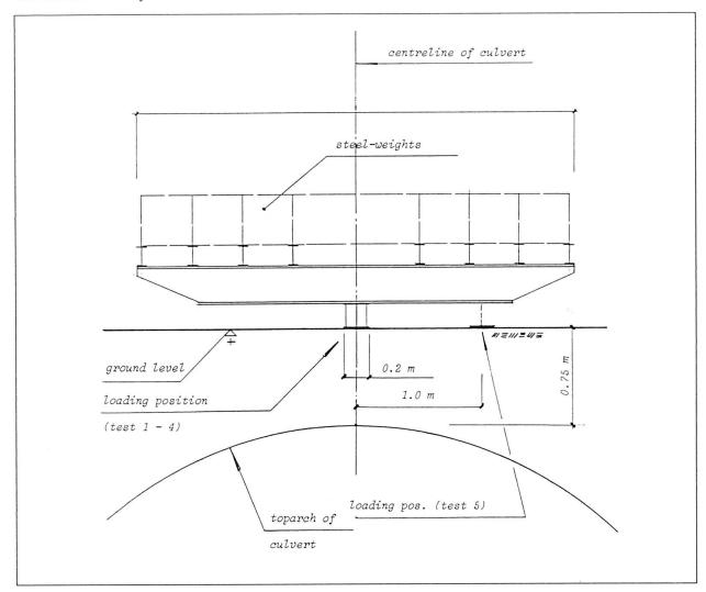
Fig. 5 Loading device for failure load tests.
