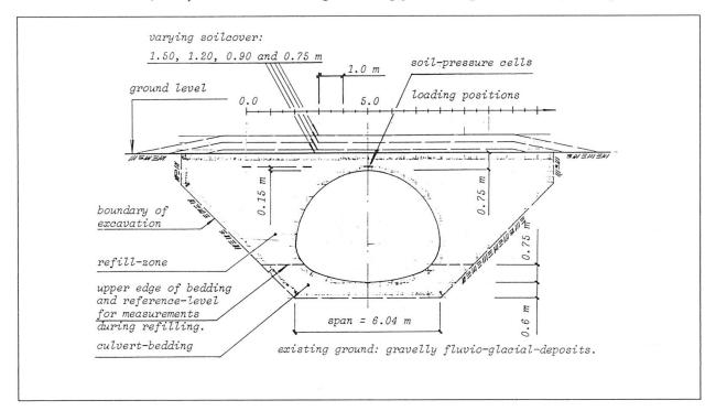
Fig. 1 Transverse section through test-culvert.
