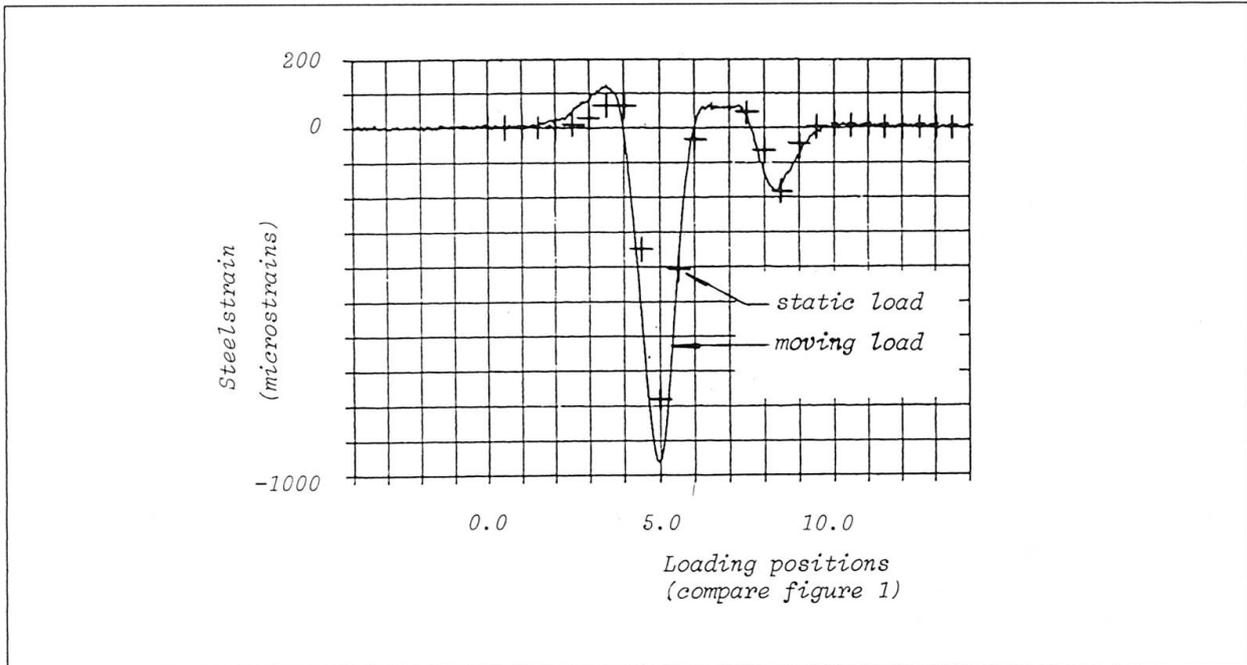
Fig. 4 Steel strains at culvert crown caused by a moving vehicle compared to steel strains caused by the same vehicle in static load positions.
