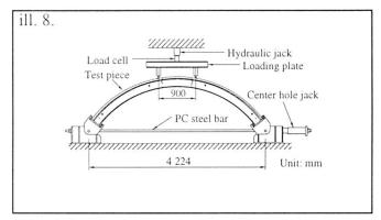
Fig. 8 Joint Bending Test Outline
