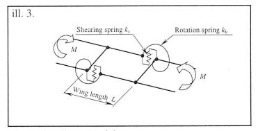
Fig. 3 Cantilever Model
