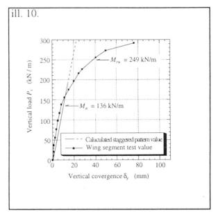
Fig. 10 Relations Between Vertical Loads and Vertical Convergence
