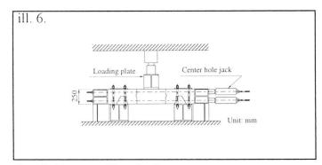
Fig. 6 Shearing Test Outline
