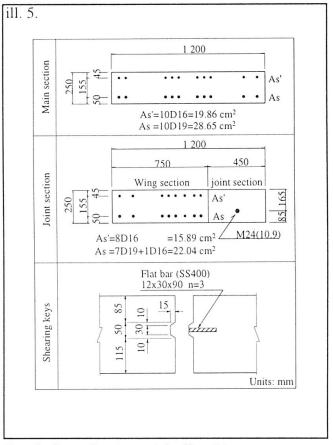
Fig. 5 Cross Sections of the Test Piece
