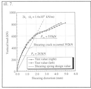
Fig. 7 Relations Between Load and Shearing Distortion
