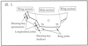
Fig. 1 Basic Construction of Wing Segments
