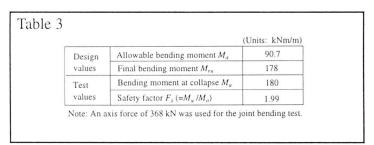
Table 3 Joint Bending Test Results
