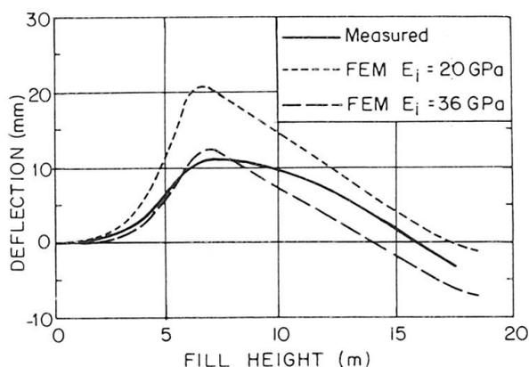
Fig. 5 : Computed and measured deflections
