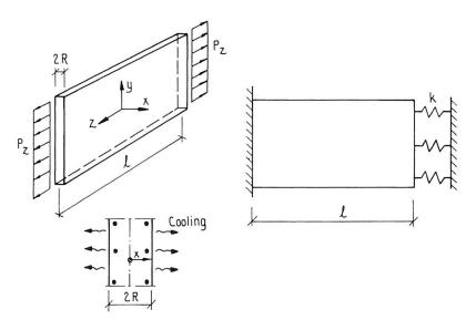
Fig.1 Geometry of the medium-thick wall.
