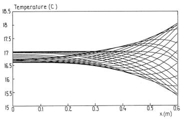
Fig.4 24 hours temperature cycle during summer in a wall with 2R=1.2 m.
