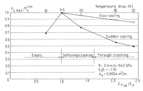
Fig.7 Force in restrained wall for strong external restraint with rapid and slow cooling.
