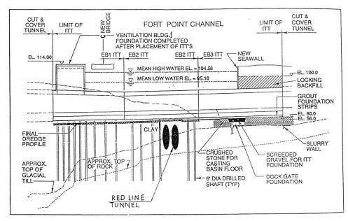
Figure 2. Longitudinal section I-90 EB in the FPC
