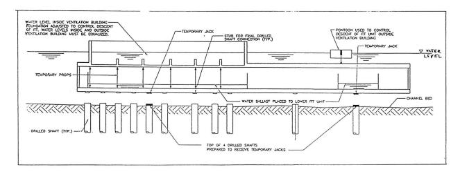
Figure 5. Immersion of the ITT with snorkel
