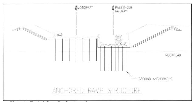
Figure 1: Typical Cross Section through ramps
