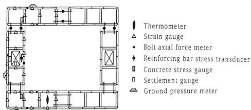
Fig. 10: Instrument arrangement plan
