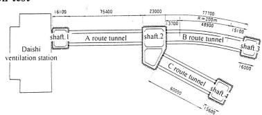
were considered; Fig. 8: Plane view of the whole of construction test plan (1) Connection pattern of individual tunnel portions (a total of four types including longitudinal and transverse connections, and two types of corner connections),
