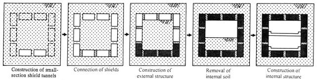
Fig. 2 Construction procedure according to the MMST method
