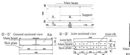
Fig. 6: Basic construction drawing of MMST steel shell
