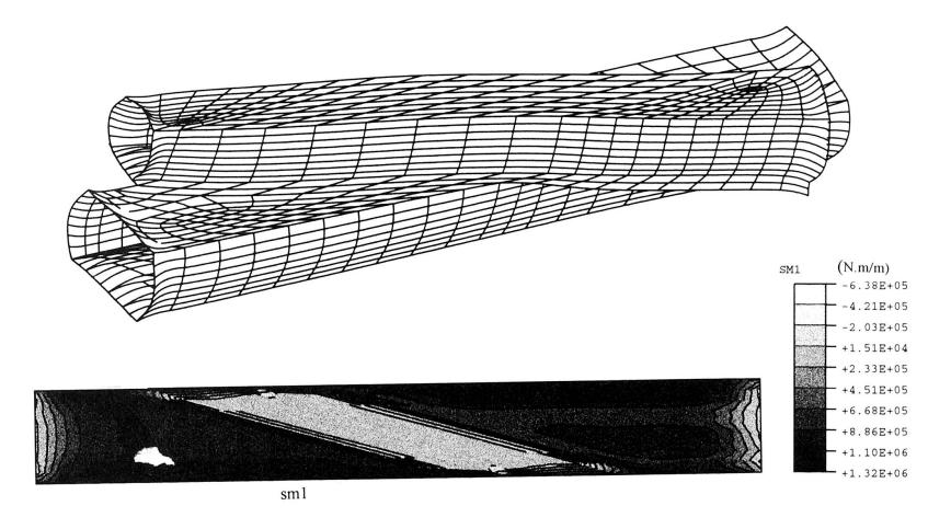
Fig. 3. Deformed structure (upper) and a moment contor map of the Intercity Tunnel roof (lower) when a load of temperature difference of 14° between the inner and outer shell-surface is applied.
