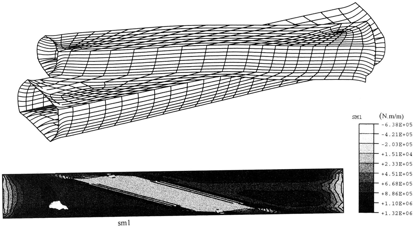
Fig. 3. Deformed structure (upper) and a moment contour map of the Intercity Tunnel roof (lower) when a load of temperature difference of  $14^{\circ}$  between the inner and outer shell-surface is applied.
