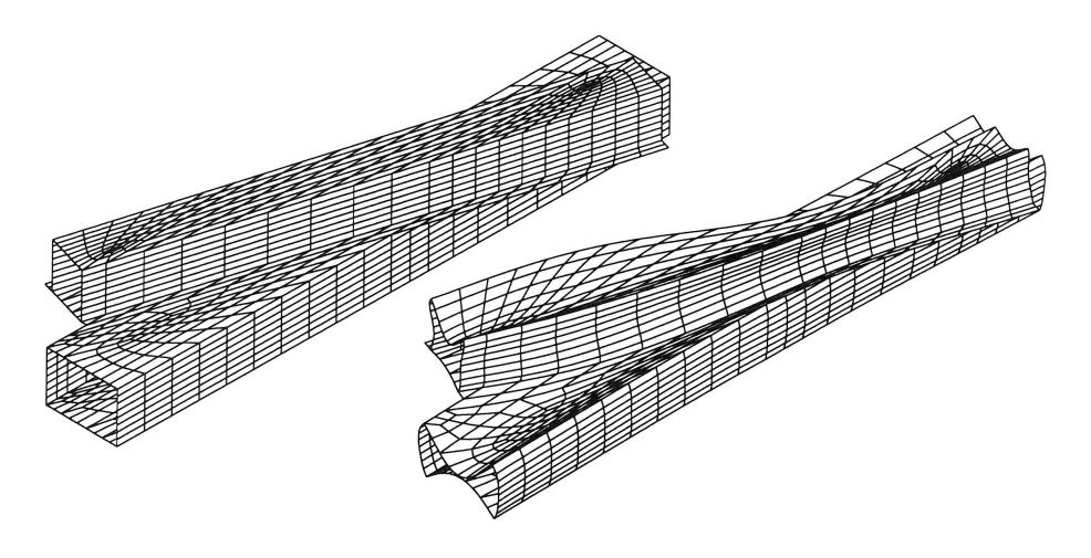
Fig. 2. Finite element mesh with 1504 thick-shell elements (left) and the deformed structure when a combined load case for damage is considered (right)
