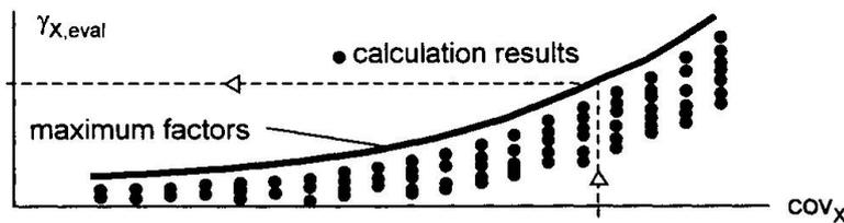
Fig.1 Schematic representation of partial safety factors for deterministic assessment,  $\gamma_{X,eval}$ , as a function of the coefficient of variation of the corresponding variable,  $cov_X$
