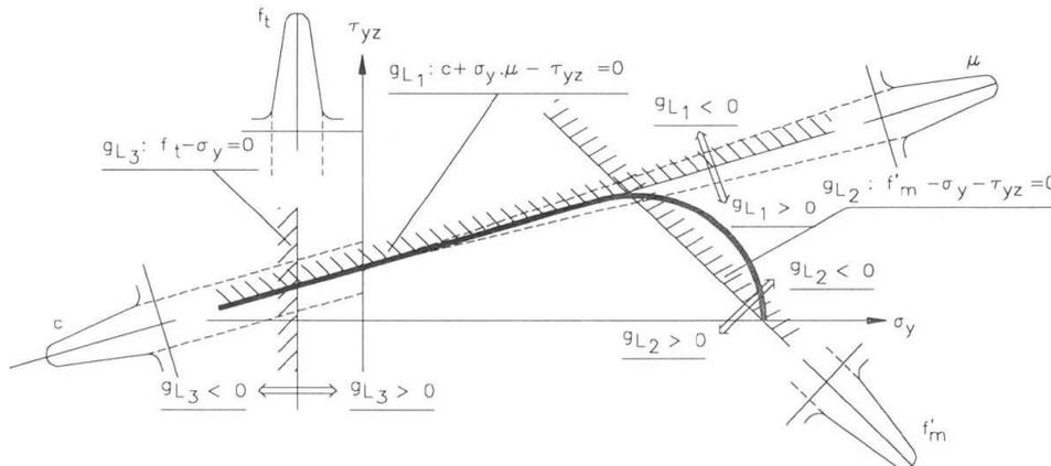
Fig. 1: Linearised "Cap-model" for unreinforced masonry shear walls
