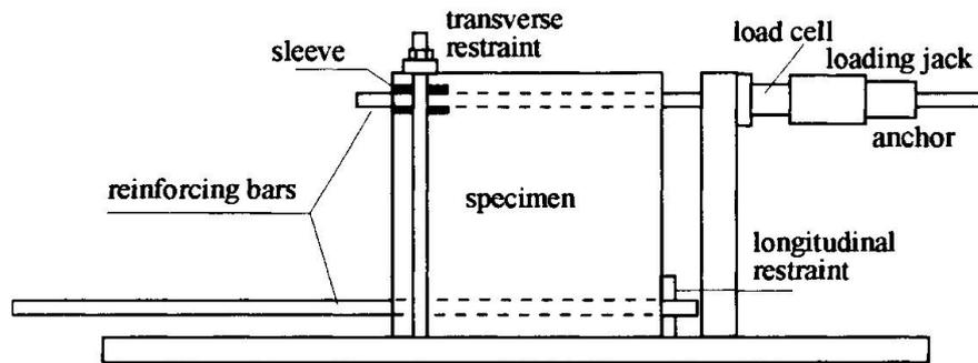
Fig 1. Bond test arrangement
