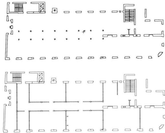
Figure 2 The plan of the existing and strengthened 1<sup>st</sup> floor
