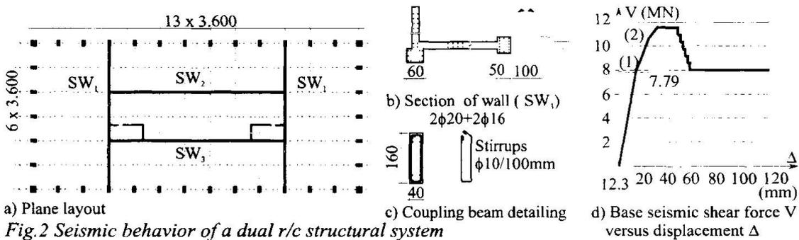
Fig. 2 Seismic behavior of a dual r/c structural system
