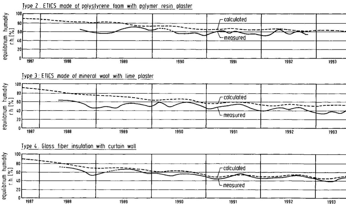
Fig. 2 Measured and calculated equilibrium humidities in the outer layers of concrete sandwich exterior walls with additional thermal insulation
