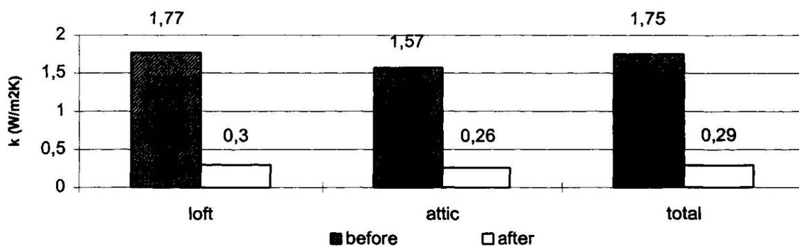
Figure 2. Average k values(W/m<sup>2</sup>K) before and after implementation of additional loft/attic insulation
