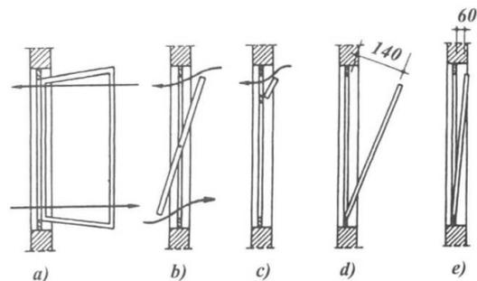
Fig. 2: Types of Window ventilation
