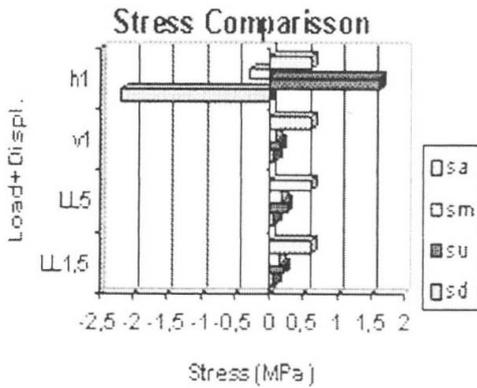
Fig 3. Comparison of the stress values caused by changes in live load (1,5 and 5 kN/m<sup>2</sup>) and abutment displacements (1cm)
