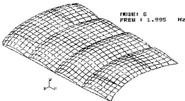
For both models, several sub-models were defined: (1) MODEL PK where the Prussian caps are the only horizontal diaphragm; (2) MODEL PK-PL are the Prussian caps with the added dead weight load due to the reinforced/concrete slab.
