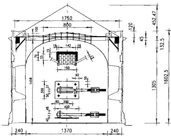
Fig. 1 Additional ties in arches including specific details
