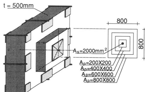
Fig. 2 The masonry panel considered with F.E.M. simulation
