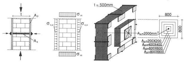
Fig. 1 Idealisation of confined masonry
