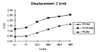
while at the same time, its additional dead load did not change basic characteristics of the main system. Average displacements were the same for all models, but their distribution along the span was different (Fig. 2 and 3). Reinforced/concrete slab contributes to the uniform displacement distribution along the span and it has activated the complete bracing system in resisting horizontal loads.
