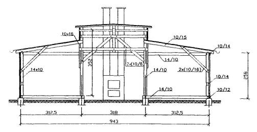
Fig. 1 The cross section of a habitable timber building
