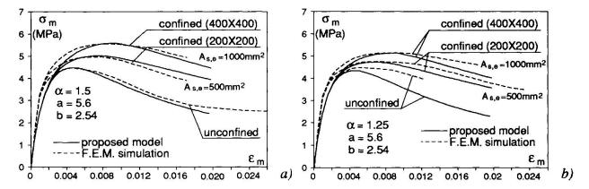
Fig. 4 Values of  $A_{s,e}$  for t=500mm (a) and 300mm (b) and corresponding behavioural curves
