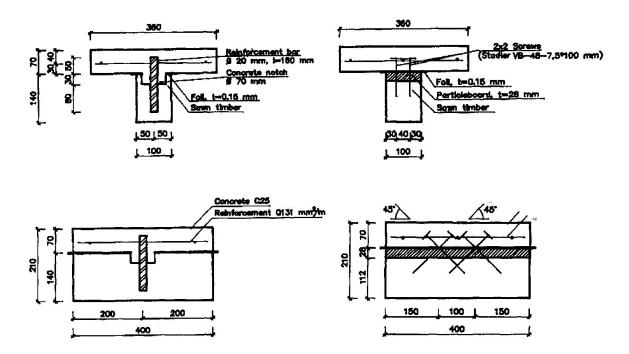
Fig. 1 Two fastener types: reinforcement bar with concrete dowel and screws at 450.
