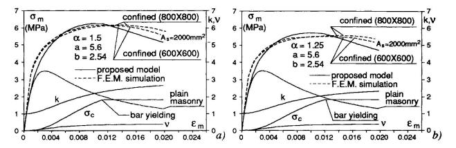
Fig.3 Fitting of the proposed theoretical model for t=500mm (a) and t=300mm (b)
