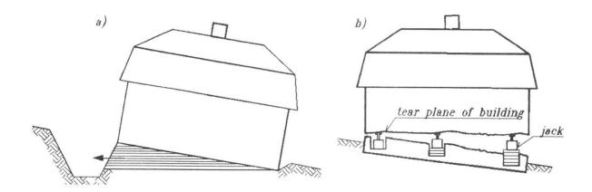
Fig. 1 Methods of buildings rectifications
