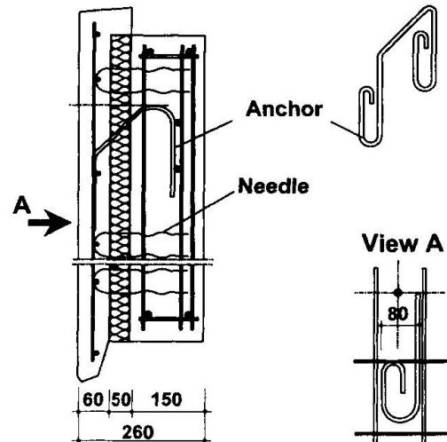
*Fig. 1: Structure of the external wall
