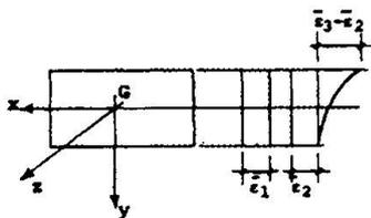
Fig. 3 Strain distribution
