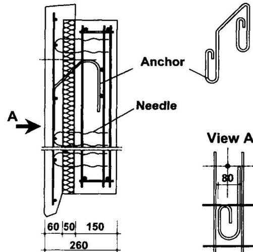
Fig. 1: Structure of the external wall
