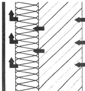
*Fig. 1 Schematic representation of back ventilated rainscreen cladding*
