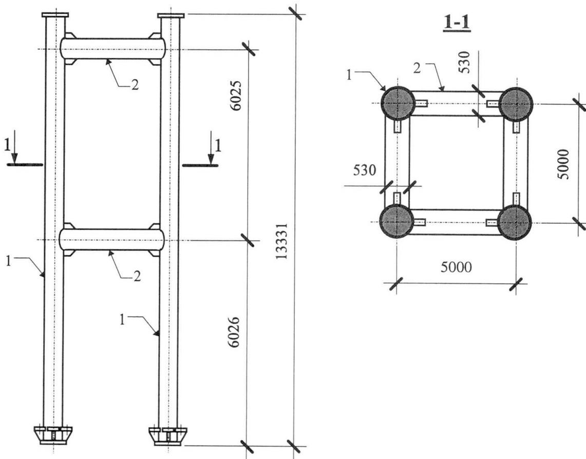
Fig. 1 Bearing of the transport gallery: 1 - strut; 2 - cross-bar
