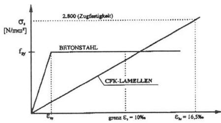
Contrary to steel, (see characteristic tension-elongation diagramme in Fig. 1), the carbon fibre strip shows an ideal elastic behaviour until break . The tension  $\sigma$  is ideally proportional to elongation  $\epsilon$  until break. The break occurs after approx. 16‰, the permissible elongation when strengthening a beam is limited to 8‰ in the Approval.
