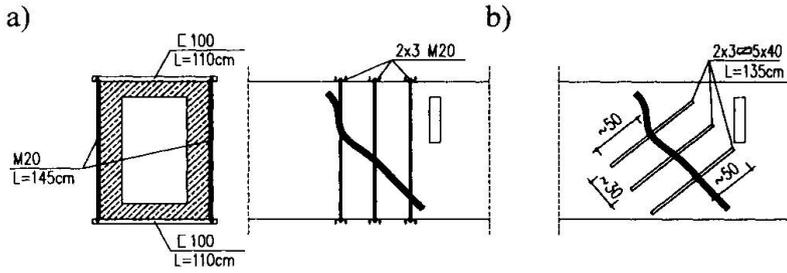
Two beams ( $b=0.20\text{m}$ ,  $h=0.30\text{m}$ ) were made as underreinforced in the shear zone. The control beam BS-0 was not repaired and the beam BS-2 was first preloaded to about 65% of its ultimate load and precracked. Next it was strengthened by steel plates  $5\times 40\text{mm}$ , bonded and
