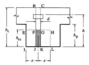
Fig. 4 Patch load for splitting failure
