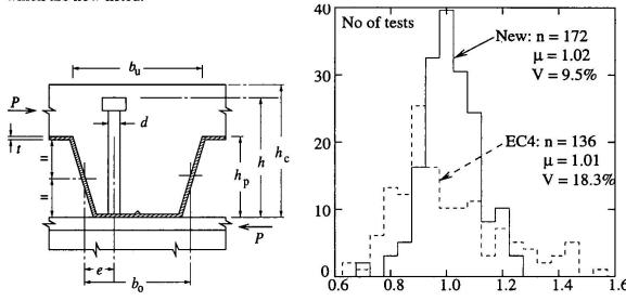
Fig. 1 Shear connector in a composite slab
