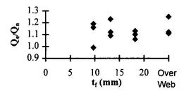
Fig. 1 Effect of flange thickness on stud strength
