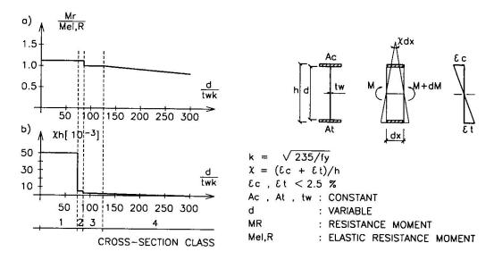
Fig. 1 Classification of cross-sections subject to bending
