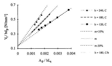
Fig. 5 Various analyses of slabs loaded according to EC4 and interpreted according to the m-k method, assuming that  $\tau(120, 350) = 0.45$  MPa, and h and  $L_s$  are varied. Coordinates are as given in EC4 [1].
