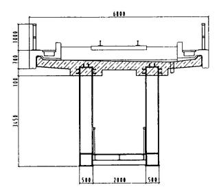
Fig. 3 Cross section of railway bridge Siemensstraße/Austria
