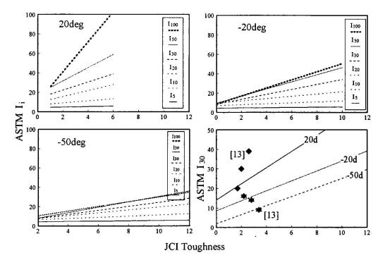
Fig. 2 Toughness correlation of T and  $I_i$  at different temperatures
