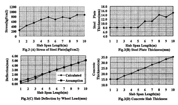
Fig.3 Calculation results of steel plate concrete composite decks.
