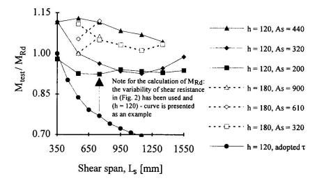
Fig. 4 Variation of bending resistance for slabs having additional reinforcement  $A_s$  when depth h and shear spans  $L_s$  are varied in slabs with  $\tau(120, 350) = 0.45$  MPa, loaded according to EC4
