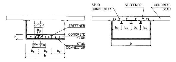
Fig. 4 Stiffened plate connected to a concrete slab
