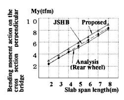
Fig 2. Design bending moments for steel plate concrete composite decks
