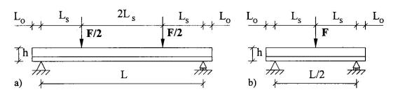
Fig. 1 Load configurations for slab tests: a) two loads according EC4 and b) single central load
