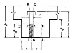
Fig. 4 Patch load for splitting failure
