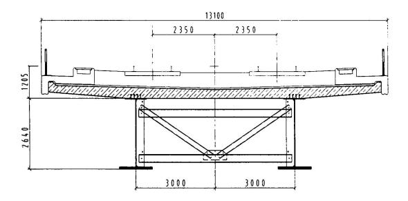
Fig. 1 Cross section of railway bridge near Melk/Austria
