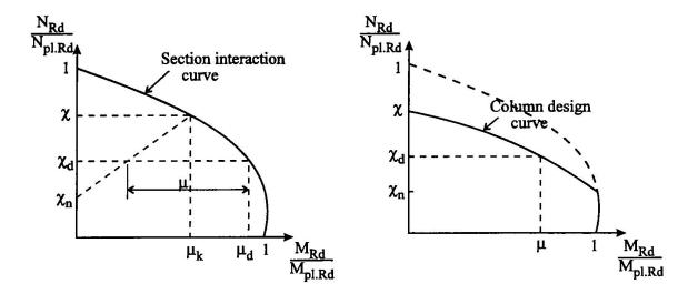
Figure 1 Design for compression and uniaxial bending
