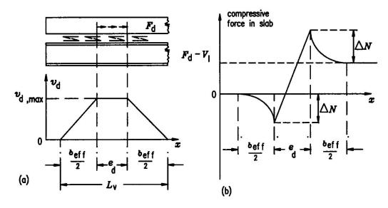
Fig. 1 Distribution of longitudinal shear force along the interface
