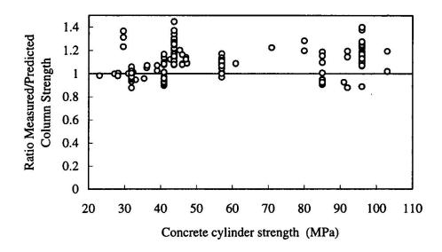
Figure 2 Column strength versus concrete strength
