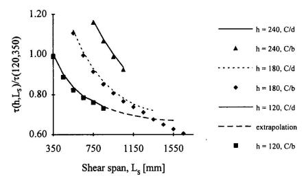
Fig. 3 Bond strength variation for strength level  $\tau(120, 350) = 0.45$  MPa for slabs with ductile (id. = d) and non-ductile (id. = b) shear connections and loaded according to EC4. Depth h and shear spans  $L_s$  in the slab are varied.
