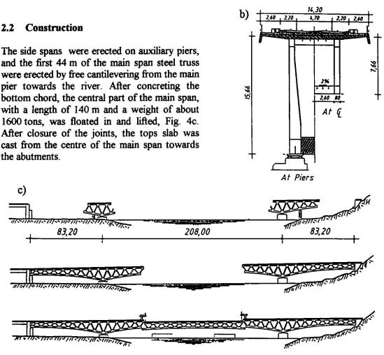
Fig. 4: Railway Bridge across Main River at Nantenbach, Germany b) Cross-section, c) Construction sequence
