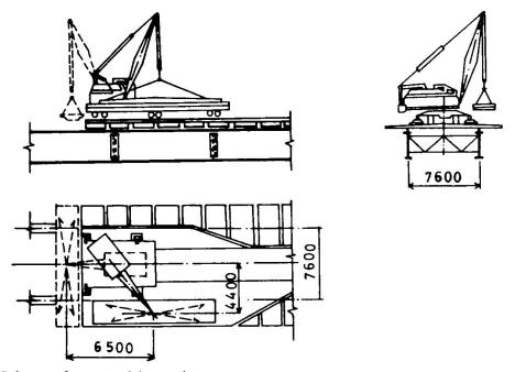
Fig. 3. Scheme of precast slab erection.
