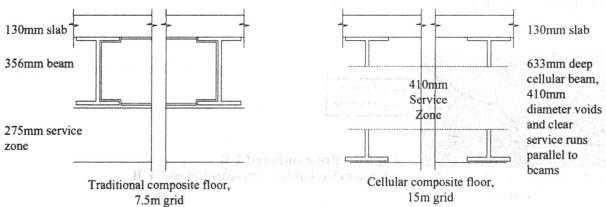
Fig 4.3 - Comparison of short span and long span floor construction.
