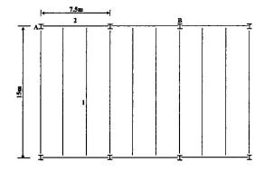
Typical short span floor. Steel S355
