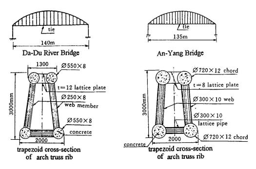
Figure 3. Da-Du River Bridge and An-Yang Bridge
