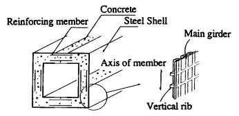
Fig. 1 Outline of steel shell for sandwich member
