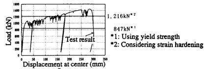
Fig. 9 Relationship between load and displacement (HB2)
