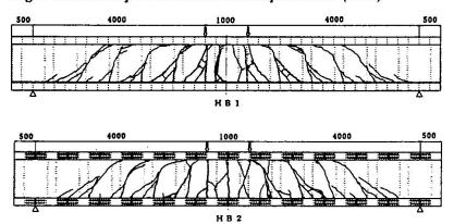
Fig. 8 Distribution of cracks (ultimate state)
