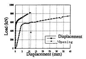
Fig. 4 Relationship between load and displacement
