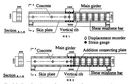
Fig. 6 Outline of specimen and arrangement of measurement points
