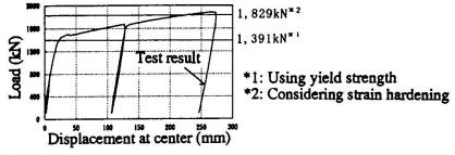
Fig. 7 Relationship between load and displacement (HB1)
