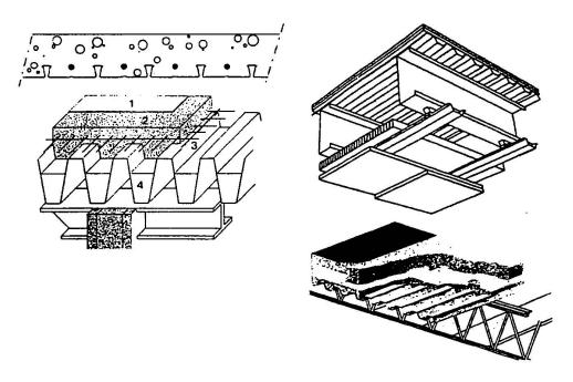
Fig. 2. Composite steel-concrete floors.
