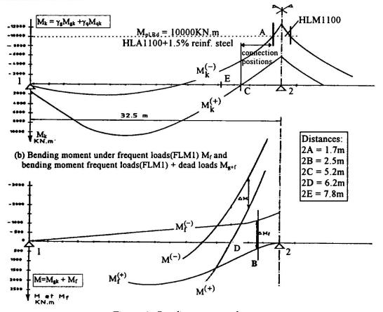
Figure 3: Bending moment diagrams
