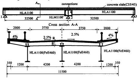
Figure 2: Composite bridge with three rolled beams
