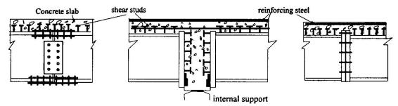
(a) Bolted cover plates connection (b) End plates connection with shear studs
