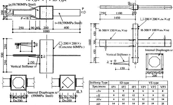
Fig. 2 Specimens of Tensile Tests
