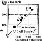
Fig. 12 Comparison in Ultimate Shear Strength of Calculated Result and Test Result
