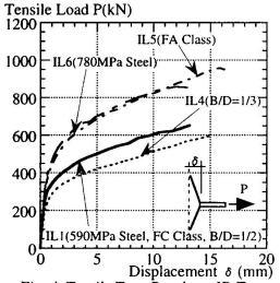
Fig. 4 Tensile Tests Result on ID Type
