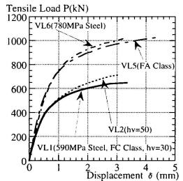
Fig. 5 Tensile Tests Result on VS Type
