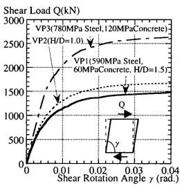
Fig. 10 Shear Tests Result on VS Type
