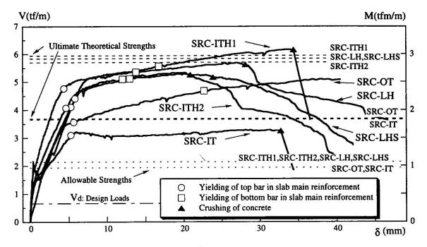
Fig. 5 Vertical load (V) versus displacement ( $\delta$ ) relation
