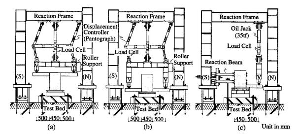
Fig. 4 Test setups for (a) ordinary T-shape, (b) inverted T-shape and (c) L-shape specimens
