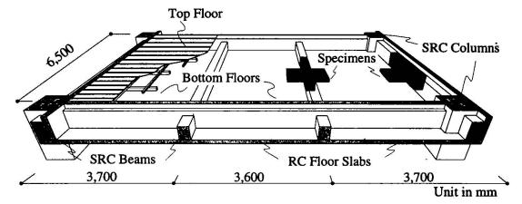
Fig. 1 Double-floor slab system
