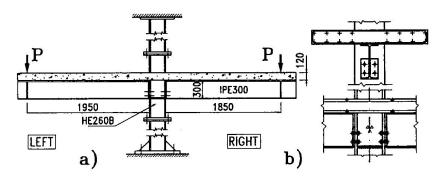
Fig. 1 The specimen (a) and the composite joint (b)
