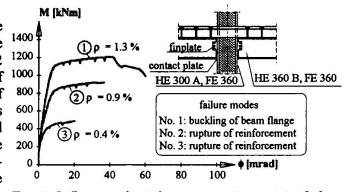
Fig. 2: Influence of reinforcement ratio on joint behaviour
