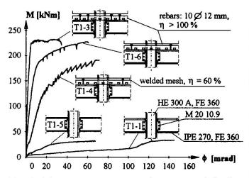
Fig. 1: Moment-rotation curves from tests with finplate connections [2]
