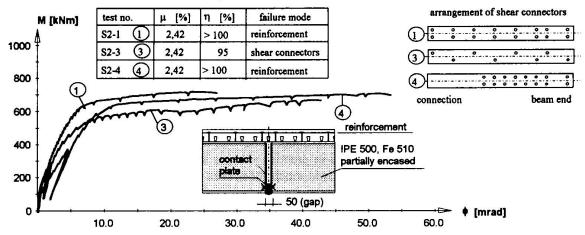
Fig. 3: Experimental moment-rotation curves
