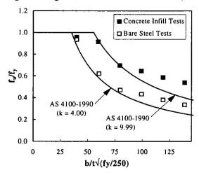
Figure 5 Strength of steel-loaded square tubes
