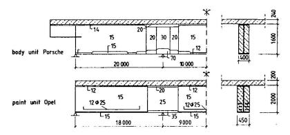
Fig. 4 Material distribution of the main girders of the body unit of Porsche and the paint unit of Opel in Rüsselsheim
