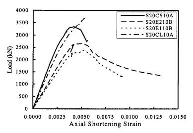
Figure 4 Load - axial strain response for S20 concrete-filled steel tubes
