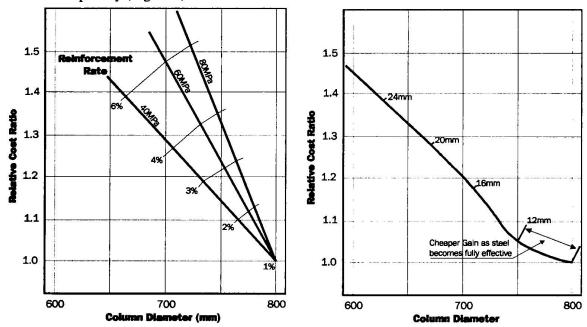
Figure 1 Relative costs for reinforced concrete columns with constant load capacity and varying percentage reinforcement
