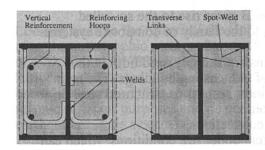
Fig. 3. Partially encased beam-column sections (Elnashai, 1996).
