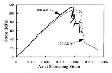
Figure 3 Stress-strain curve for high strength concrete from cylinder tests.
