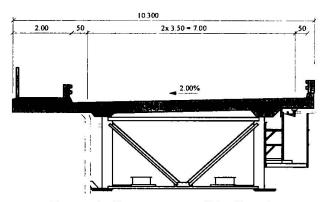
Figure 6: Cross-section of Nordbrücke
