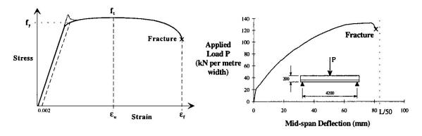
(a) Stress-strain curve from coupon testing Figure 6 Tensile testing of G550 sheet steels
