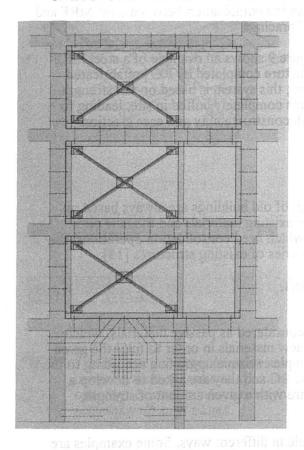
Fig. 5. RC frames with steel bracings.
